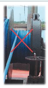
LEFT: Line installed incorrectly on working side of winch drum! On working side of winch, only wrap a single layer of line (8 wraps). Working part of line should come off end of wraps, not from the middle as shown
