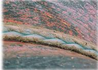
Line installed on storage side of winch drum. Cross-overs prevent AmSteel-Blue from divina between layers and getting stuck during deployment.
